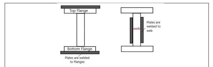
4. Compare the bending strength of the two beams having different cross section (one is of hollow rectangular cross section and other is of I-section). I-section is formed by welding of back to back webs of two 'C' sections whereas hollow rectangular section is formed by welding of face to face top & bottom flange of two 'C' sections as shown.
